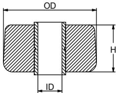
Available in two insert size options. Please specify hole size: 5/8" to fit 1/2" bolt or 1/2" to fit 3/8" bolt
