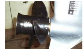
Fig. 3 Failure to install gearcase adapter ring leaves gap that causes excessive ventilation, poor performance.
