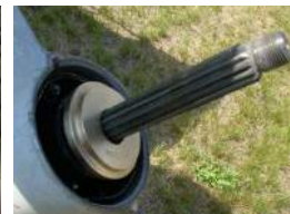
Fig. 7 The forward thrust washer is tapered and will nest with the taper on the propeller shaft. When properly installed, the part number will be visible.
