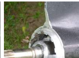
Fig. 7 The forward thrust washer is tapered and will nest with the taper on the propeller shaft. When properly installed, the part number will be visible.
