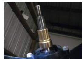
Fig. 8 The forward thrust washer MUST be installed first. Failure to install a forward thrust washer will cause gearcase damage and potential injury.
