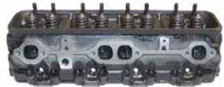
18-4485 CYLINDER HEAD ASSEMBLY Fits: 5.7L V-8 GM (1987-95) with press in rocker arm studs with 12 intake manifold mounting bolts- (4 inside intake manifold bolts at 23 degrees), center mount valve covers
