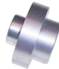
18-9843 CLAMP PLATE Replaces: Mercury Marine 91-43559 Description: Holds preload while checking backlash and bearing preload on Bravo One and Two drive units.
