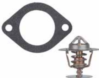
23-3664 THERMOSTAT KIT Replaces: Kohler 249970, 29963 Temperature Rating: 190° Fits: 8E, 10E, 12.5E, 12.5CF, 15C, 16CF, 20C, 10 EG, 13 EG, 13 EGZ, 15 EG, 15 EGZ
