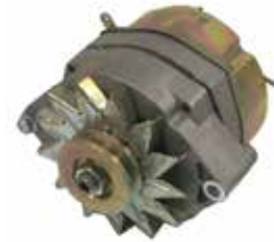
18-5957 ALTERNATOR (3-Wire) (No Core) (68 AMP) Replaces Mando, Motorola and original equipment Delco. Uses same electrical connections and mounting method. Equipped with fan and drive pulley. Replaces: 78477, 78403A2, 92497A3. • SAE J1171
