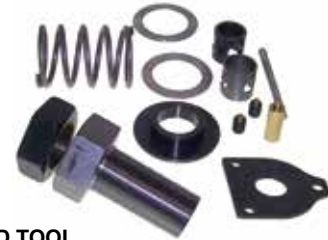
18-9806E SHIFT CABLE TOOL Replaces: Mercury Marine 91-12037 Description: Installs and removes shift cables on MC-I, R-MR, Alpha One, Alpha One/Gen II drive units. Use with 18-2190 and 18-2190E cables.
