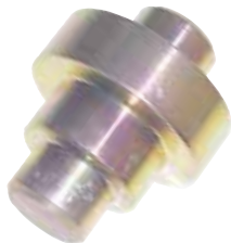
18-9846 SEAL DRIVER Replaces: Mercury Marine 91-44110 Description: Installs oil seals in water pump base on Alpha One and Alpha One/Gen II drive units and outboards.
