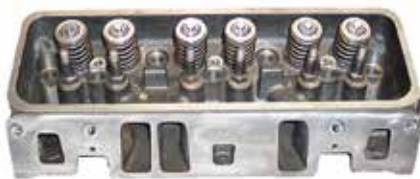
18-4491 CYLINDER HEAD ASSEMBLY Replaces 4.3L Vortec V-6 (1996-Up) with screw in rocker arm studs (non-adjustable valve train), 8 intake manifold mounting bolts, center mount valve cover. NOTE: not for use with engines using factory roller rocker arms.
