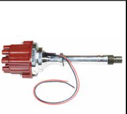
18-5479 ELECTRONIC DISTRIBUTOR Fits: GM V-8 engines-reverse rotation
