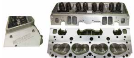
18-4502 CYLINDER HEAD High Performance Aluminum cylinder head sold in pairs only. This utilizes a 185cc intake runner/62cc exhaust runner and 2.02/1.60 stainless valves placed in a 72cc combustion chamber. Fits: 5.7, 6.2L GM small block V-8
