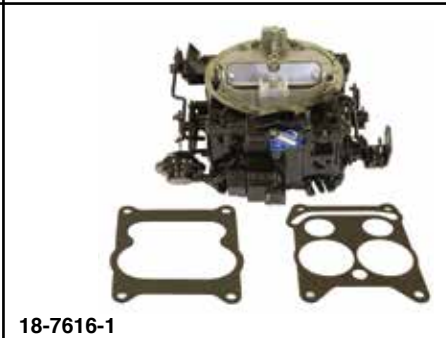
18-7616-1 CARBURETOR (REMANUFACTURED) 4 Barrel - Rochester Replaces: Mercruiser 1347-8288A1, 1347-804626R02, Rochester 1708563, 17057287, 17059287, 17059290, 17080560
