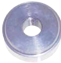
18-9839 BEARING CUP DRIVER Replaces: Mercury Marine 91-38918T Description: Installs bearing cup in top cover of drive shaft housing of MC-I, R-MR, Alpha One drive units and outboards.
