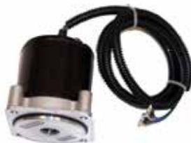
18-6783 TILT/TRIM MOTOR Replaces: 64E-43880-00-00, 64E-43880-01-00 2-wire ring terminal connection 4-bolt mount For: 115-225HP (1997-2002)
