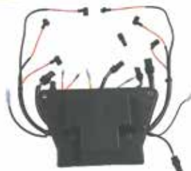
18-5893 POWER PACK Replaces: 586667, 584037, 586217, 583476 For: V-4 & V-8 6700 rpm limit
