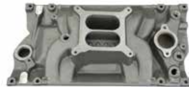
18-7628 INTAKE MANIFOLD Small-block GM with vortec cylinder heads with brass lined water jackets
