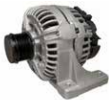
18-6953 ALTERNATOR Replaces: Volvo 3803645, 8602629, 8602710, 14 8676496, 98, 8676499 Fits: Diesel D3 Models
