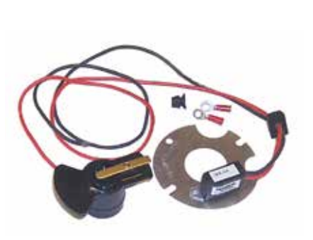
18-5288 HI-PERFORMANCE ELECTRONIC CONVERSION KIT Fits: Most Prestolite V-8 Distributors with snap down cap
