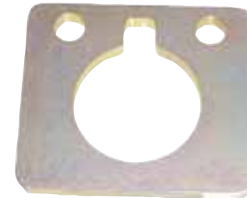
18-9843 CLAMP PLATE Replaces: Mercury Marine 91-43559 Description: Holds preload while checking backlash and bearing preload on Bravo One and Two drive units.
