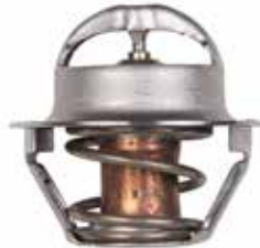
23-3602 THERMOSTAT Replaces: Westerbeke 37387 Temperature Rating: 140° Fits: 4.5 BCG(60Hz)/3.75 BCG(50Hz), 7.0 BCG(60Hz)/5.0 BCG(50Hz), 7.0 BCGA(60Hz)/5.0 BCGA(50Hz)
