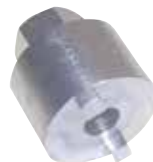
18-9817 SHIFT SHAFT BUSHING TOOL Replaces: Mercury Marine 91-31107T Description: Removes and installs the shift shaft bushing in the gear case of MC-I, R-MR and Alpha One drive units and outboards.
