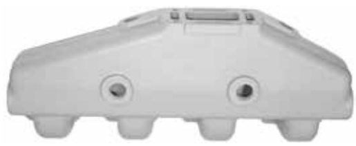
18-1898 MANIFOLD Port & Starboard Replaces: Barr CHVA-1-84, Marine Power 0991-110 Fits 454 cu.in. GM big block V8 engines Use with: Exhaust Manifold Gasket: 18-0418 *For Exploded View - See Pages 556-557
