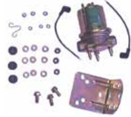
18-7333 ELECTRIC FUEL PUMP UNIVERSAL 12V, 72GPH at 5.75 PSI, 1/4" NPSF for 3/8" hose, for use with gasoline and diesel fuel.
