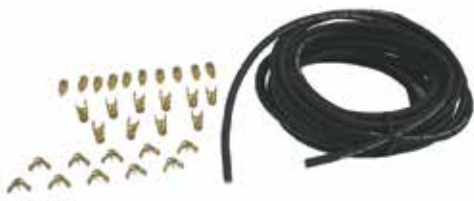
18-5225 SPARK PLUG WIRE KIT Kit includes 25 ft. Roll of 7 MM Hypalon Ignition Wire With a Metallic Core and a Large Assortment of Three Different End Fittings to Fit Outboard Motors.
