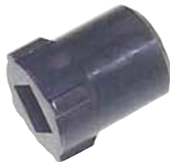
18-9844 TAPERED INSERT TOOL Replaces: Mercury Marine 91-43579 Description: Installs tapered insert retainer into water inlet hose on all Bravo drive units.
