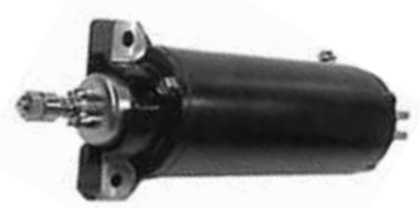
18-6283 STARTER Replaces: 50-8331535, 50-898265008 For: Mercury 2.5 DFI(1999 and up), 200HP V6 DFI(1996-99), 225HP V6 DFI(1998 and up), 3.0L V6(1999 and up) 9 tooth drive gear
