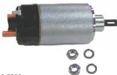
18-5806 SOLENOID Replaces: 834520 BOSCH 0331-302-050, 0331-302-081, 0331-302-085, 0331-302-581, 0331-302-585 For starters with aluminum nose. Slot in end of solenoid shaft is 13/32" long.
