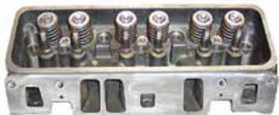
18-4491 CYLINDER HEAD ASSEMBLY Replaces: MerCruiser 938-827178 1 Replaces 4.3L Vortec V-6 (1996-Up) with screw in rocker arm studs (non-adjustable valve train), 8 intake manifold mounting bolts, center mount valve cover. NOTE: not for use with engines using factory roller rocker arms.
