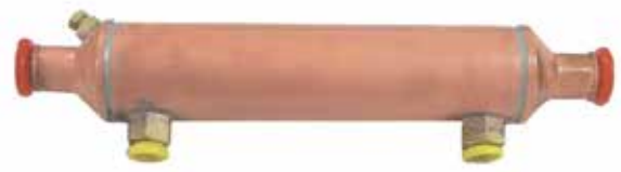
18-2589 TRANSMISSION OIL COOLER • 1" Water Hose Connection • 9" Tube Bundle Overall Length • Approximately 12" • Oil-6 GPM MAX Water 25 GPM MAX • Shipped bare metal, ready for primer and factory paint finish.
