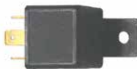
18-5704 POWER TRIM RELAY Replaces: 876037 20 Amps Resistive 15 Amps Inductive Single Pull 5 Terminal For: AQ270, 280
