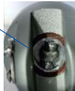
A Dogbone blocks the halyard in the swivel
