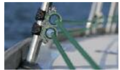
With the different Facnor fairleads, the lines run clearly on the deck Above : articulated fairlead (left handside) et twin fairlead (right handside)
